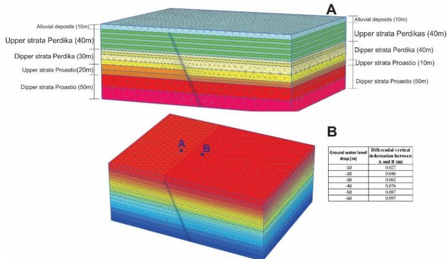
**Figure 2. A. Simplified 3D simulation model of the site at the village of Valtонера, B. The results of deferential vertical displacements due to the level drop of the aquifer.**
