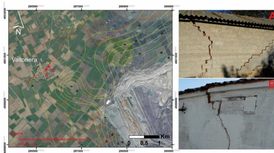
**Figure 1. Distribution of the surface ruptures at the Valtонера village in relation with drawdown contour lines.**
