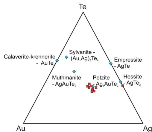
**Figure 2. Ternary Au-Ag-Te diagram of typical Au, Ag and Au-Ag tellurides (blue rhombs), and Au-Ag and Ag tellurides (red squares) from the intermediate volcanoclastic conglomerate of the Perama Hill epithermal Au deposit.**
