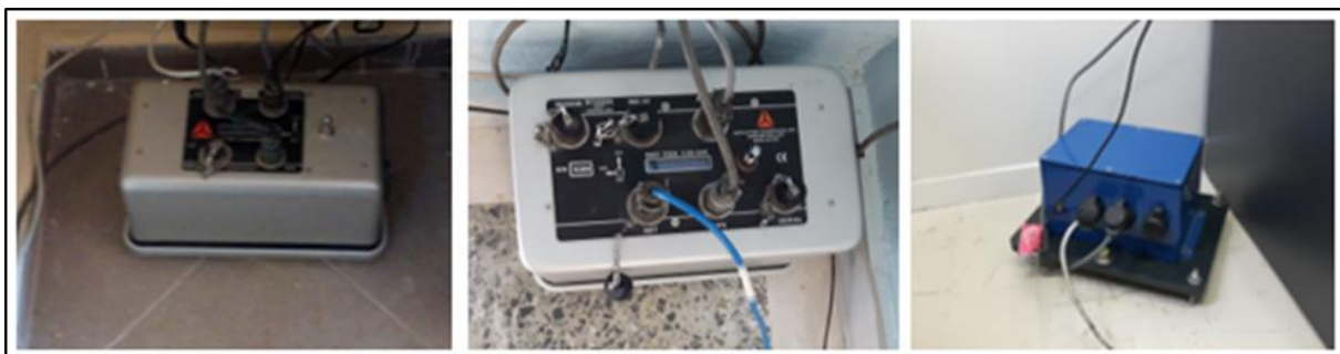
Figure 1. The three types of accelerometer installed for the SGM network, the Ref Tek 130 ANSS/02(left) the 130 SM (middle) and the GSense (right).
