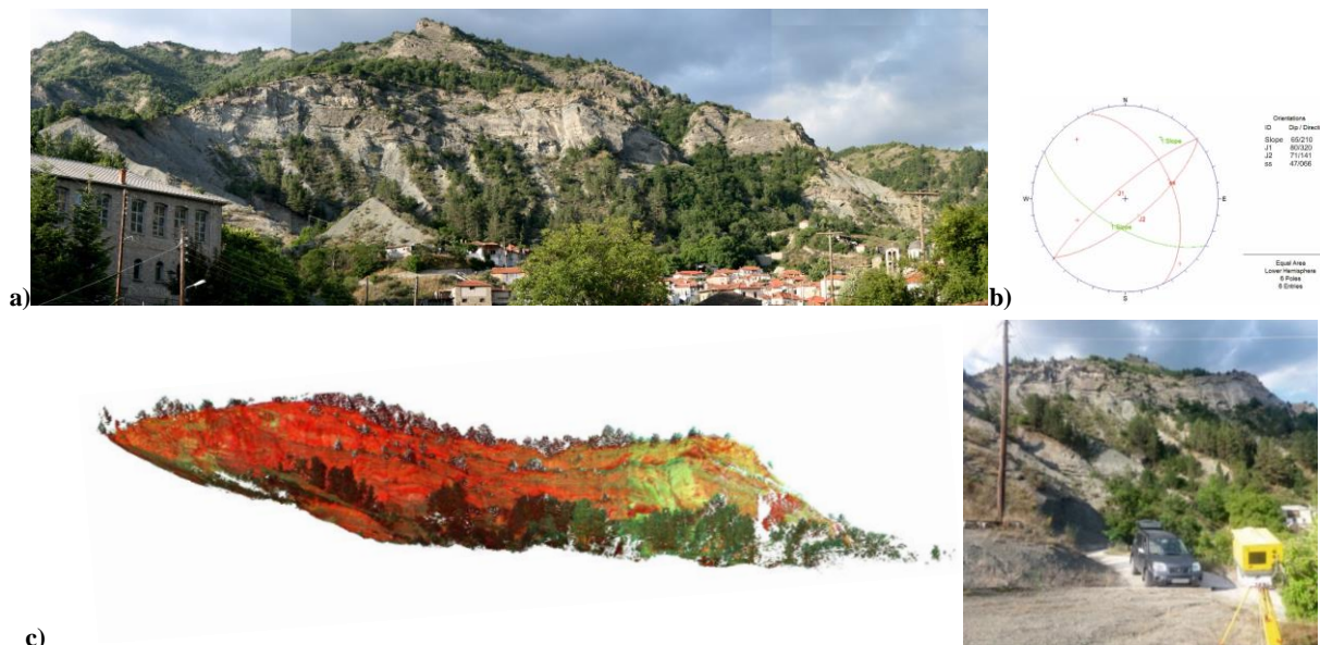
Figure 1. (a) Face log of the slope to SW, (b) Major planes of the rock mass in Schmidt projection, (c) Resulting point cloud from LiDAR scanning
