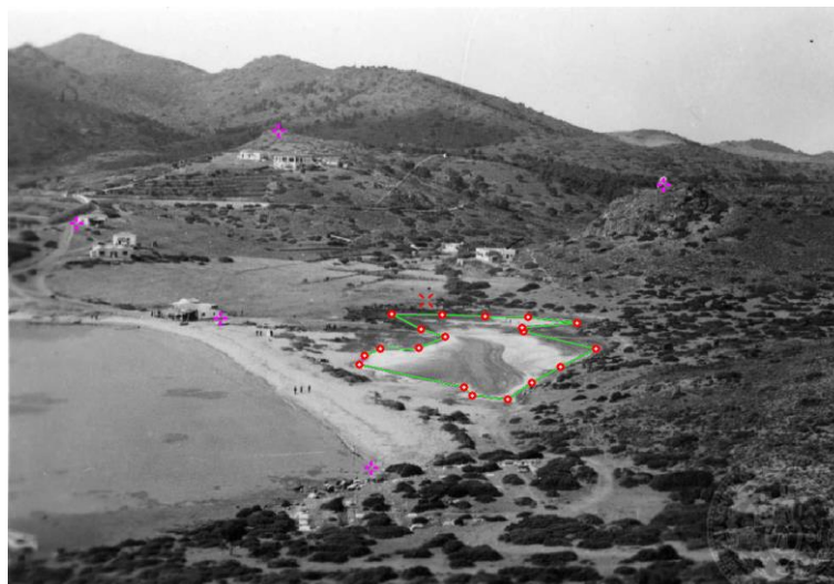
Figure 1. Digitizing of a landform from historical photograph within the environment of Monoploting tool.
